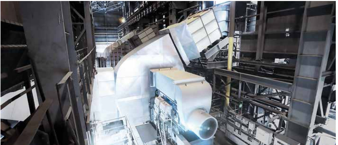
Wear protection, gas tightness and a low danger of caking are essential factors for industrial fans in the cement production process.
